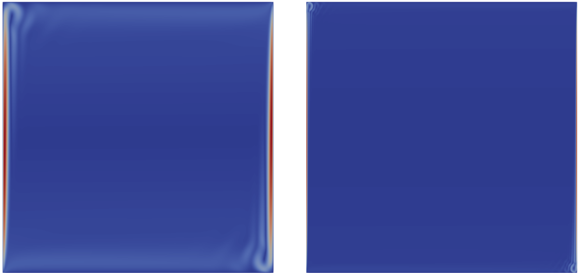
Figure 15: Profiles of flow velocity magnitude at Ra_c for \log_{10}Pr = 0.205 (left) and \log_{10}Pr = 0.225 (right) for the insulating floor and ceiling boundary conditions. Note the abrupt change in scale of the corner flows between the two plots. The scale bars are not shown but the peak speed in the right-hand plot is \approx 20 times that in the left-hand one. The difference in Ra_c between the two plots is more than two orders of magnitude.
