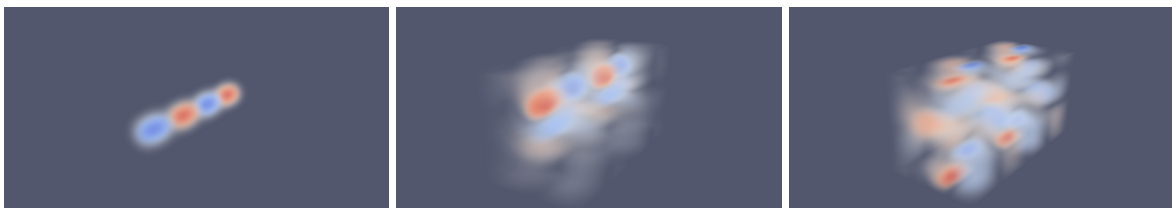
Figure 3: Plots showing the time-evolution of an initial Gaussian density profile modulated by a sinusoid in the axial direction, in a 3-D implementation of the 2-D Hasegawa-Wakatani equations. Periodic conditions are used in all dimensions. This output either precedes the appearance of turbulence or lacks the physical and / or numerical conditions needed to generate turbulence.
